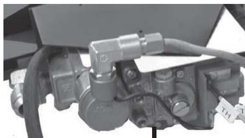
G46 burner showing remote-control valve layout under heat shield
