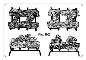
CAUTION: Burn hazard. Logs will remain hot for some time after use. You must maintain the log layout as shown to ensure proper operation of your log set. If you need to reposition any log to maintain the proper layout, use heat-resistant gloves or allow logs adequate time to cool before handling.
