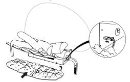
Install the Mirage<sup>™</sup> Flame Panel by inserting the bottom edge into the tabs between the back log and grate log assemblies.
