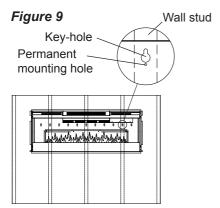
a minimum of two wall studs available for mounting.
