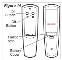
the plastic insulator strip out from between the remote casing and battery cover (Figure 14).
