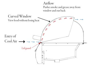
The Magic View Window has been designed for the natural air movement in the grill to keep it clean. Cool air enters the closed oven through the small gap (created by the lid guards) at the front of the grill; then it follows the contour of the hood, exiting the back. This airflow keeps smoke and grease away from the window, reducing build-up and making it easy to clean.
